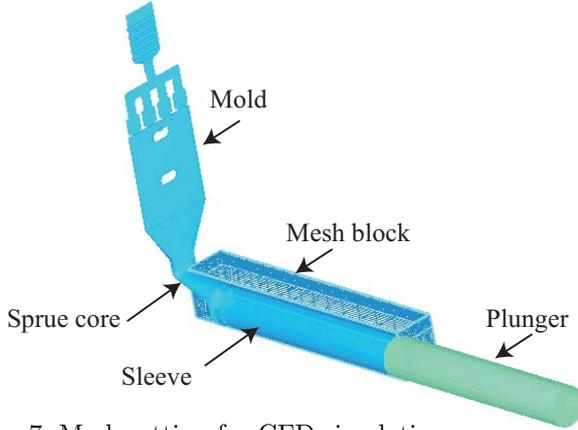
Fig. 7. Mesh setting for CFD simulation.
