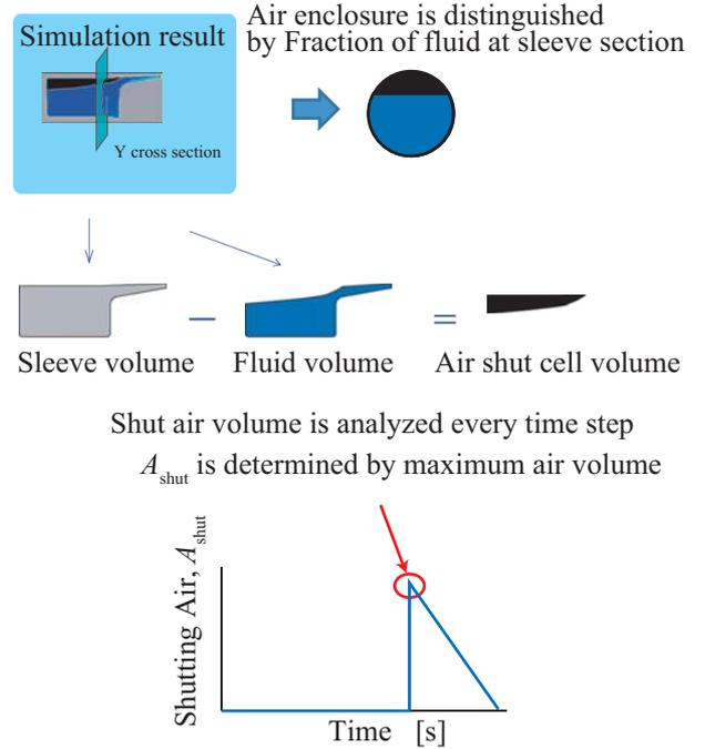
Fig. 8. Distinction of the shutting the air in the sleeve.
