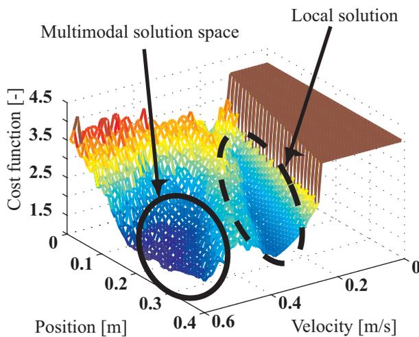
Fig. 10. Relationship of air entrapment with plunger velocity and switching position as calculated with CFD simulator.
