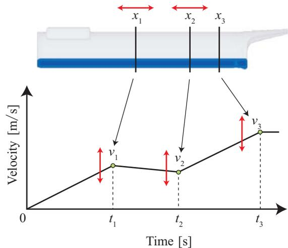
Fig. 6. Die-casting simulation model using 5 variables.
