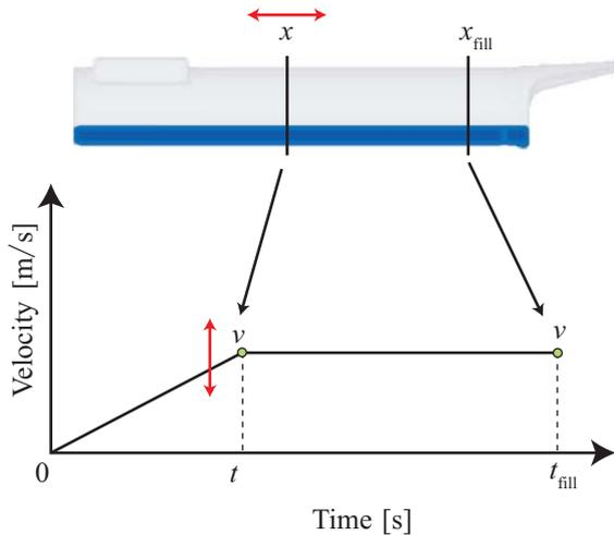
Fig. 9. Die-casting simulation model using 2 variables.
