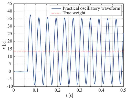
Fig. 2. Practical oscillatory waveform of the load cell
