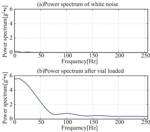
Fig. 3. Power spectrum function  $P_1(f)$  of white noise and after the vial is loaded, by performing FFT
