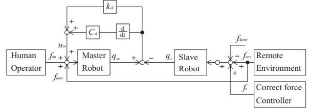
FIGURE 3. Block diagram in motion condition 2
