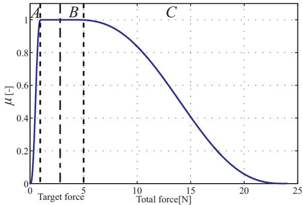
FIGURE 5. Bell shaped trajectory for  $\mu$  controller
