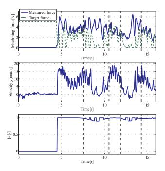
**FIGURE 7**. Experimental result of machining with proposed bilateral control and constant machining value method
